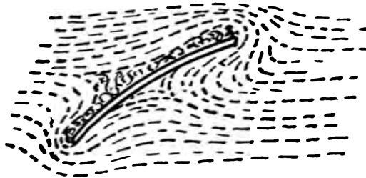
FIG. 18.—Resistance of air to curved aeroplane.
